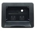
TBUS-3US-22 provides an extremely simple, affordable and elegant multi-connection boardroom solution with a tilt-up lid. TBUS-3US-22 is fast and easy to install and comes preassembled with an inner frame, 2 power sockets, 1 cable pass-through insert and 1 blank insert
